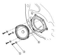
• Install the speaker by using included speaker cable ⑥.
