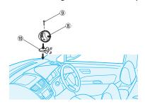
Adjust the spacer ® into the preferred direction for the correct sound output, then adhere using the included cushion ®.
