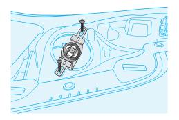
• Install the tweeter into the vehicles genuine dashboard position by using the vehicle pre-fitted screw.
