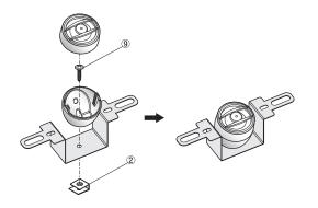
Tighten tweeter and adapter by using the included nut ② and screw ③.
