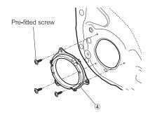
• Install the adaptor 4 into the vehicle by using pre-fitted screw.
