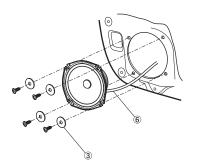
• Install the speaker into the vehicle by using vehicle pre-fitted screw and included speaker cable (6).
