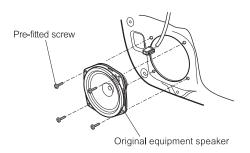
• Take pre-fitted screw, connector, and original equipment speaker out.
