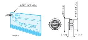
• Drill a hole of  $\,\phi$ 42 mm (1-5/8" Dia.) in the preferred position of door trim.
